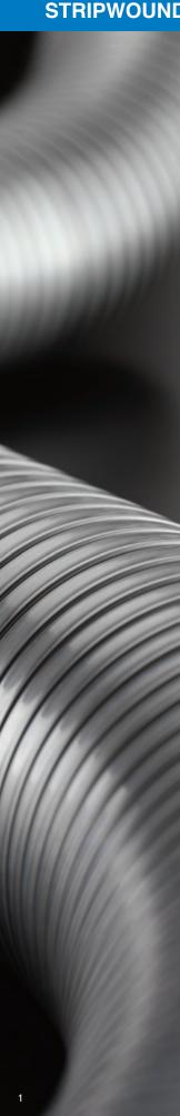
Stripwound metal hose is a rugged product made from a strip of steel that is profiled and continuously wound around a mandrel to form a hose. Hose Master's proprietary manufacturing process yields an extremely consistent and balanced profile that maximizes strength and flexibility. Stripwound hose is used as a guard, exhaust hose, and for the transfer of dry bulk materials.
