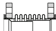
TD - Telescoping Drop-in These liners are used for large axial movement and can be removed and cleaned.
